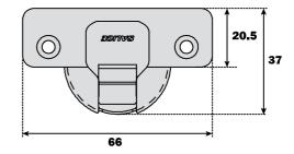
Constant "L" value of 0.7 mm (it does not change during side adjustment).
